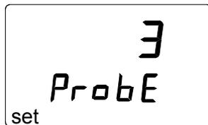
Select **PROBE TYPE 3** with buttons ▲ (number up) or ▼ (number down) and turn the indicator off. Turn it on again by pressing the ON/OFF button. After a few seconds, the relative humidity and temperature readings appear automatically on the display. **The HMP45D cannot be used with the HMI41 indicator as the passive temperature signal results in error messages on the HMI41.**
