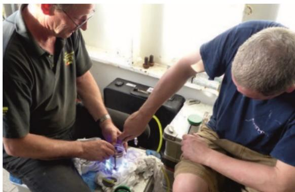
▲ HyBIS engineers Dave and Russ filling the beacons with oil so that the high pressure at the ocean floor does not cause the glass to break. Photo: B. J. Murton
