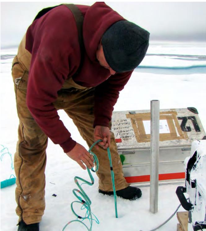
A chain of temperature sensor chips is lowered through the ice in the Canadian Arctic. The chains use satellite modems to transmit profiles of data from the sea to improve understanding about the sea ice.
